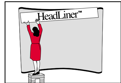
Hang headers, HeadLiner, or Velcro® graphics last. For detailed instructions on HeadLiner, refer to the lighting section of this guide.
